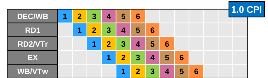
Targeted pipeline stream (with vertical transfer)
